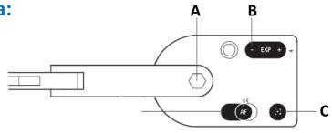
**A: SWIVEL HEAD** – In addition to the joints of the stand, you can further customize your image by swiveling the camera 270° (180° clockwise and 90° counterclockwise).
